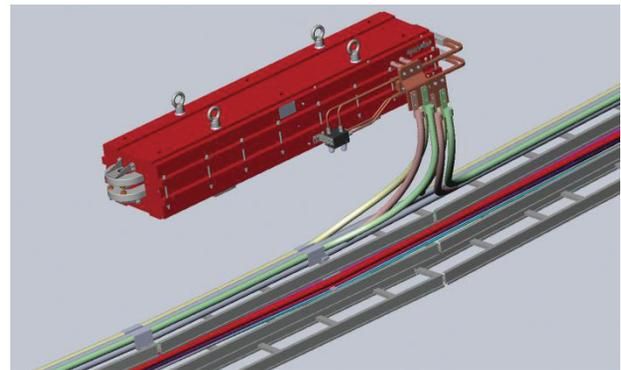
Figure 1: The booster dipole magnets connect with the dipole cable.
