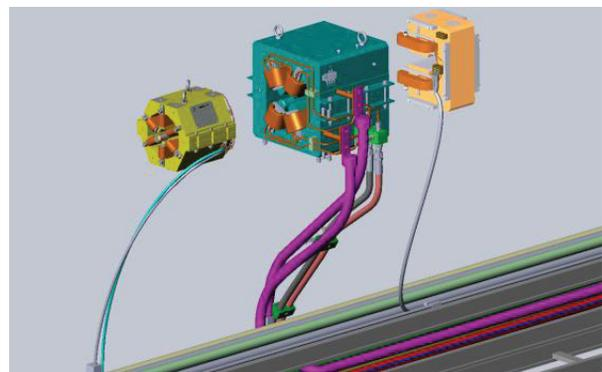
Figure 2: The booster quadrupole, sextupole and corrector magnets connected with cables.
