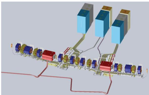
Figure 4: The cabling from the CIA room to the magnets.
