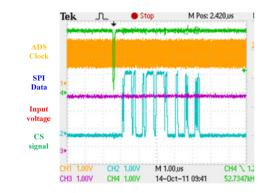
Figure 4: Timing of ADS1278 data converter.
