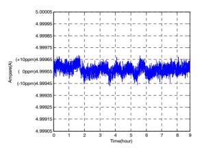
Figure 10: Stability of output current of the corrector magnet power converter within 8 hours
