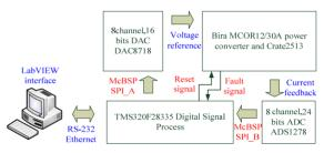
Figure 1: The structure of digital control interface card and the LabVIEW control program.
