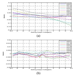
Figure 7: The capture current signal of ADS1278EVM converter (a) the linearity error without correction (b) the linearity error with correction.
