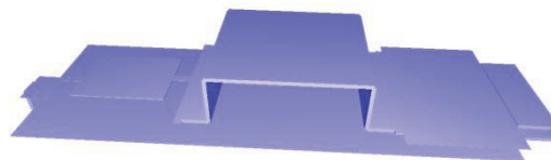
Figure 4: A FastHenry model of a single current branch of a layer of the inductive adder.
