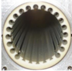
Figure 4: 19 beam screen conductors, each with a sphere.
