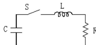
Figure 1: Simply equivalent circuit.
