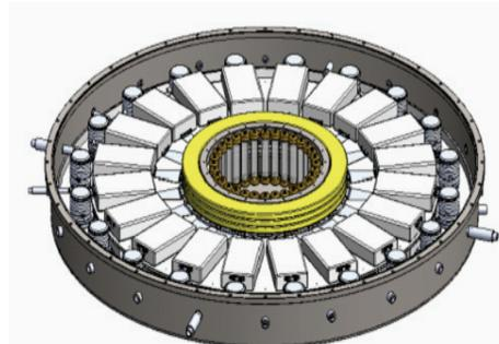
Figure 3: 500KA/150ns LTD stage sans top flange.
