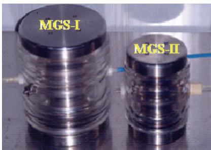
Figure 2: Photo of the multi-gap multi-channel switch.
