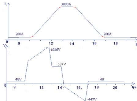
Figure 3: pulsed wave of dipole power supply in HIRFL-CSRm.
