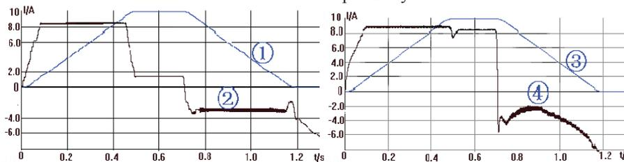
Figure 4: output-current and regulator waveforms of the two power supply.
