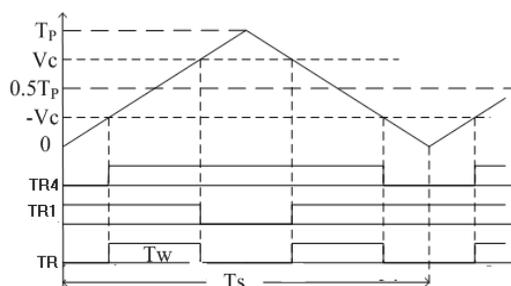
Figure 2: driving waves of the H-bridge chopper.
