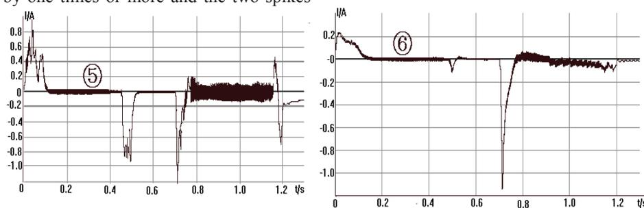
Figure 5: curve for following error of the current.
