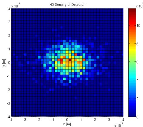
Figure 4: H<sup>0</sup> distribution at the detector 3.5 m downstream the laser.
