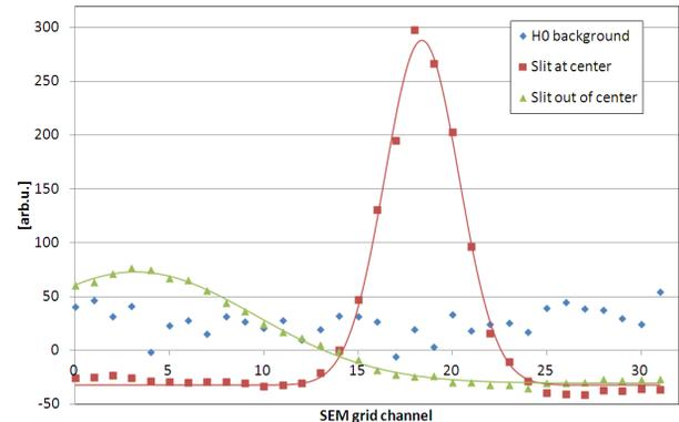
Figure 6: First results from 3 MeV test stand with 200  $\mu\text{m}$  slit.
