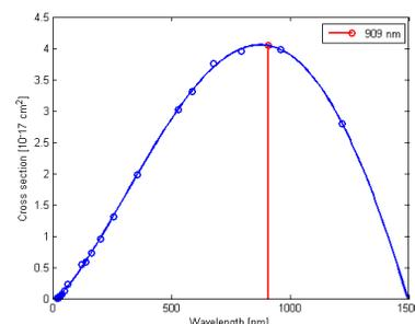
Figure 2: Photo neutralization cross-section [1]; in red: Lorentz shifted 1064 nm laser at beam with 160 MeV.
