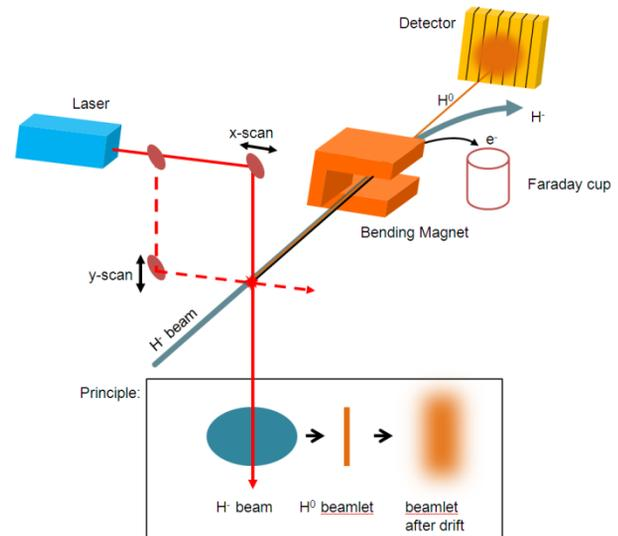
Figure 1: Concept of the laser emittance meter.
