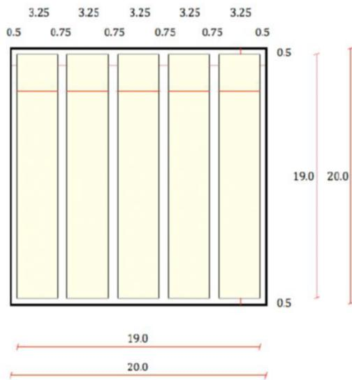
Figure 5: Polycrystalline diamond detector with 5 strips (sizes in mm) [4].
