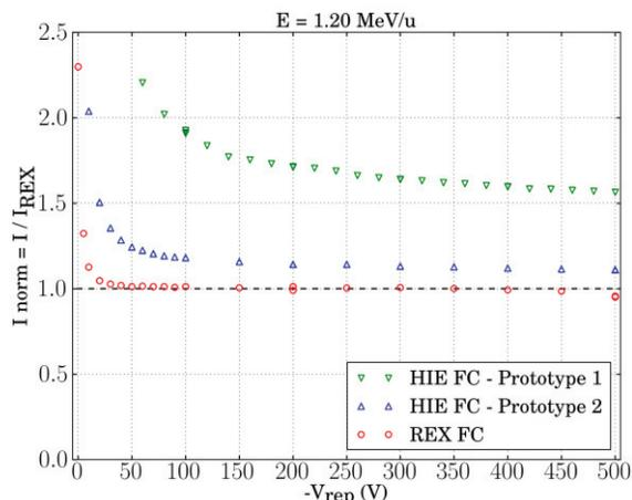
Figure 6: Normalized current as a function of the repeller potential for ions with energy  $E = 1.20$  MeV/u.
