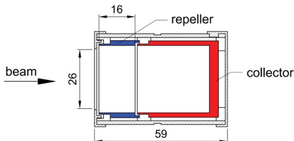
Figure 1: Layout of a standard Faraday cup, used at ISOLDE. Dimensions in mm.
