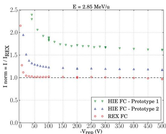
Figure 7: Normalized current as a function of the repeller potential for ions with energy  $E = 2.85$  MeV/u.
