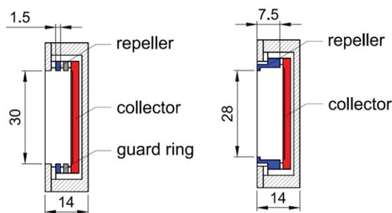
Figure 2: Layout of the prototype Faraday cups. Dimensions in mm. Left: Prototype 1. Right: Prototype 2.
