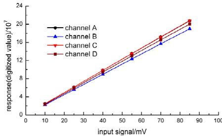
Figure 4: Channel response under different input signal
