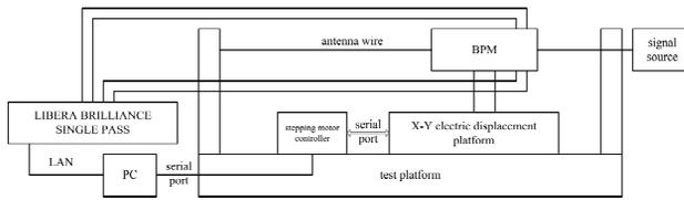
Figure 3: Calibration test stand.
