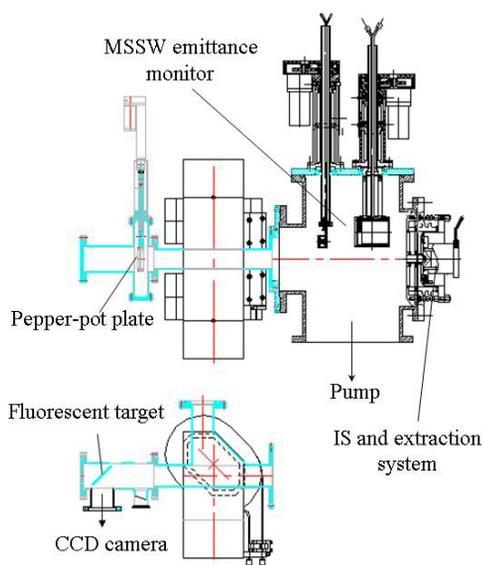
Figure 4: Mechanical design of measurement device.
