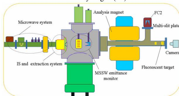
Figure 1: Layout of the IS test bench.
