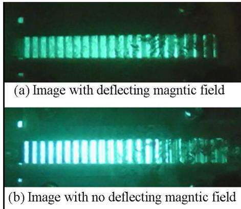
Figure 2: Image of quartz fluorescent target.
