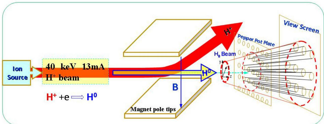
Figure 3: Outline of beam emittance monitor based on neutral beam fluorescence.
