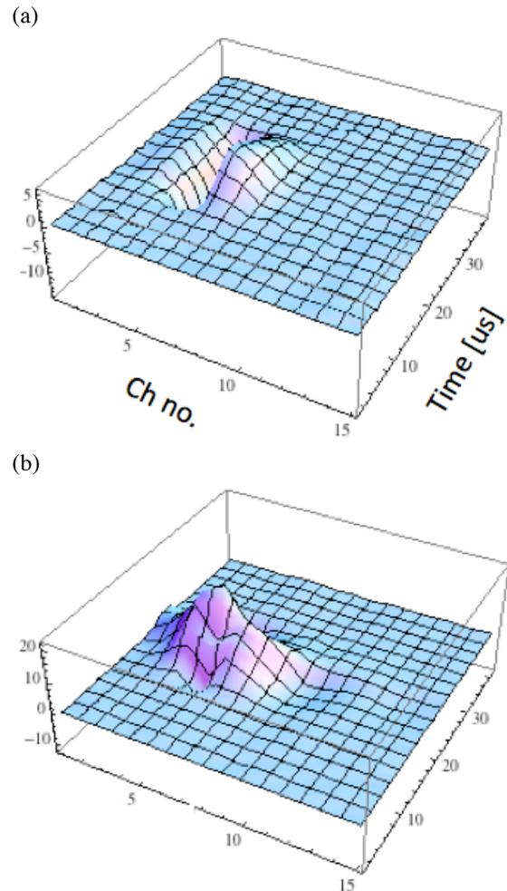
Figure 6: Measured data by our test model. (a): deflectors are off. (b): deflectors are on ( $\pm 10 \text{ V}$ )
