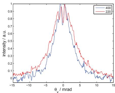
Figure 4: Central vertical cuts normalized to the maximum intensity for the (220) and the (400) reflection. The data were obtained from the measurements shown in Figs. 2 and 3 for the beam size  $\sigma_x = 45.7 \mu\text{m}$ ,  $\sigma_y = 42.9 \mu\text{m}$ , and  $\theta_x = 0 \text{ mrad}$ .
