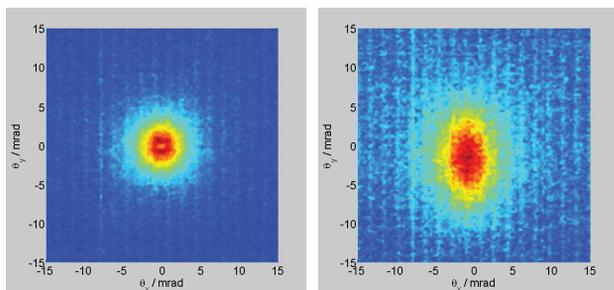
Figure 3: Measurement of the PXR angular distribution for the (400) reflex. Left: beam size  $\sigma_x = 45.7 \mu\text{m}$  and  $\sigma_y = 42.9 \mu\text{m}$ , right:  $\sigma_x = 44.7 \mu\text{m}$  and  $\sigma_y = 796 \mu\text{m}$ .
