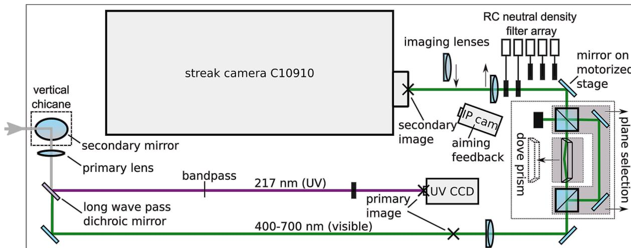
Figure 3: Optics layout roughly to scale. A dichroic mirror separates the UV from visible synchrotron light. The latter is collimated and guided into a plane selecting section. Variable imaging lenses determine the magnification ratio.
