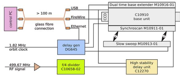
Figure 6: Streak camera block diagram.
