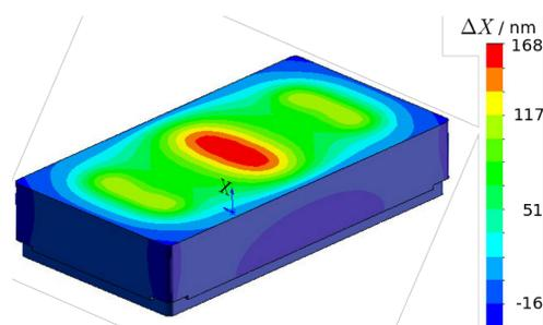
Figure 2: FEM analysis showing the deformation of the mirror surface when irradiated and water cooled [1].
