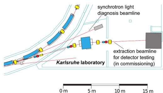
Figure 1: External diagnostic beamline for synchrotron light analysis.
