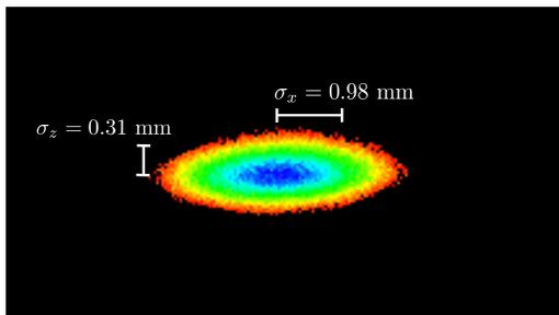
Figure 5: The beam profile in the UV range at 1.2 GeV. The measurement was performed with a non-dichroic mirror.
