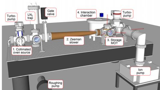
Figure 1: The layout of the PSI cold electron source.
