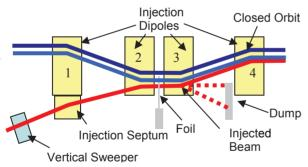
Figure 1: Schematic layout of the existing 70 MeV ISIS injection system.
