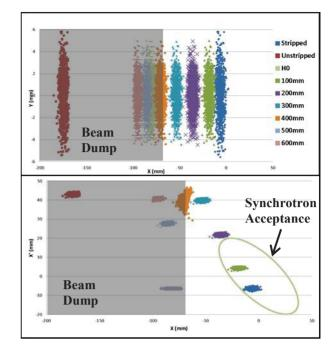
Figure 6: Real space (top) and horizontal phase space (bottom) distributions of fully, partially, delayed and unstripped particles at the end of the injection region. The shaded area illustrates the beam dump.
