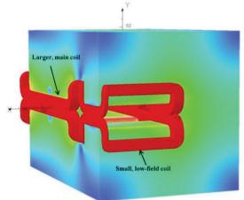
Figure 2. Initial design of a two-stage injection septum.
