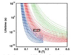
Figure 4: Stark state and lifetimes for n=5 (green), n=6 (red) and n=7 (blue). The region of interest is highlighted.
