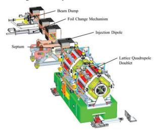
Figure 3: Initial CAD model of the lattice quadrupoles and new injection region.
