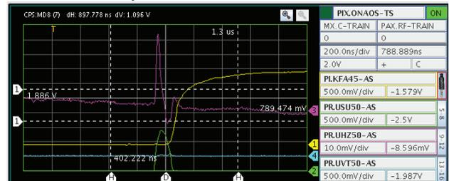
Figure 2: For the kicker timing  $t=0$  only part of the bunch (red curve) is kicked due to slight fluctuations of the kicker delay and bunch phase.
