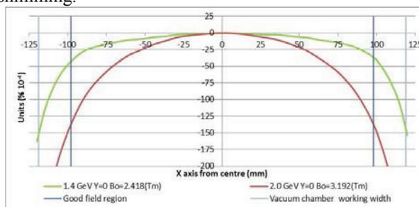
Figure 6: Field homogeneity of the integrated B field along the horizontal axis  $[10^4 \cdot (\int B_{y(x,0,z)} - B_{y(0,0,z)}) / B_{y(0,0,z)}]$ .
