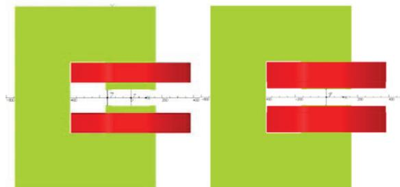
Figure 5: Present coil configuration (left), proposed coil configuration (right).
