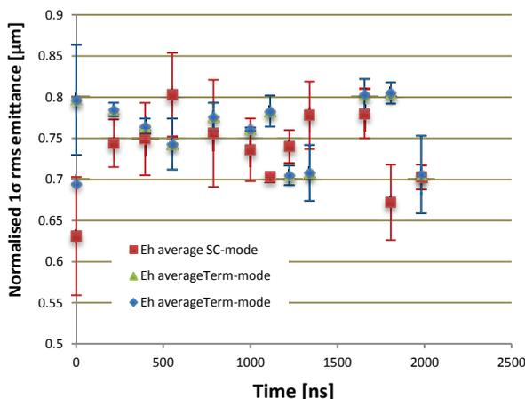
Figure 1: Horizontal emittance measurements for the injection kicker in terminated and short-circuit mode.
