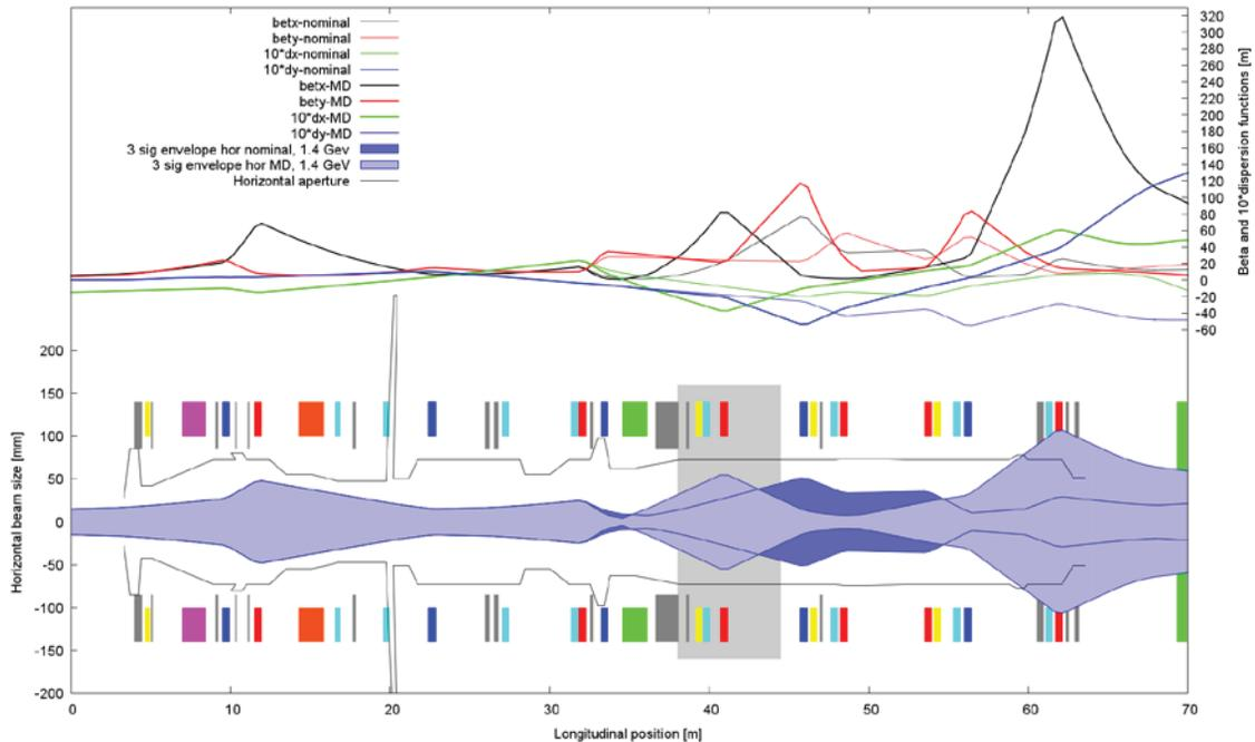
Figure 3:  $3\sigma$  beam sizes of the nominal and measurement beam (lower part) and the optics for both cases (top part).
