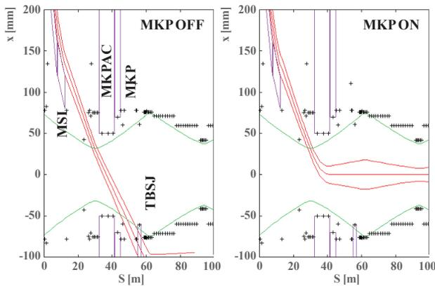
Figure 2: Present 17.1 GeV/u Pb<sup>82+</sup> ion injection into the SPS with  $\pm 5 \sigma$  beam envelopes.
