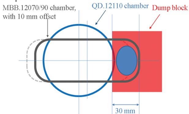
Figure 4: Dump block upstream of Q.12110, and downstream of the offset dipoles MBB.12070 and 90.
