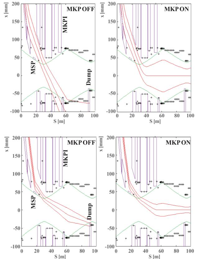
Figure 3: New 17.1 GeV/c/u Pb<sup>82+</sup> ion injection (top) and 14 GeV/c p+ injection, into the SPS with  $\pm 5 \sigma$  beam envelopes.
