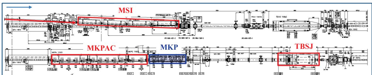
Figure 1: The two half-cells of the present SPS injection system, shown septum MSI, kickers MKPAC and MKP, and beam dump TBSJ.
