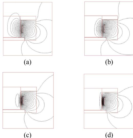
Figure 4: RF magnetic field in different ionization rates.  $x$  is the ionization rate of the plasma in the driver. (a),  $x=0$ ; (b),  $x=0.001$ ; (c),  $x=0.01$ ; (d),  $x=0.1$ .
