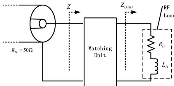
Figure 2: Equivalent circuit of the RF Load.
