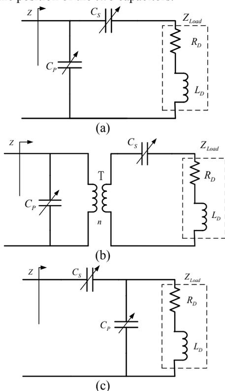
Figure 5: Three kinds of impedance-matching networks. (a) is the first scheme call No.1. (b) is the first scheme call No.2. (c) is the first scheme call No.3.
