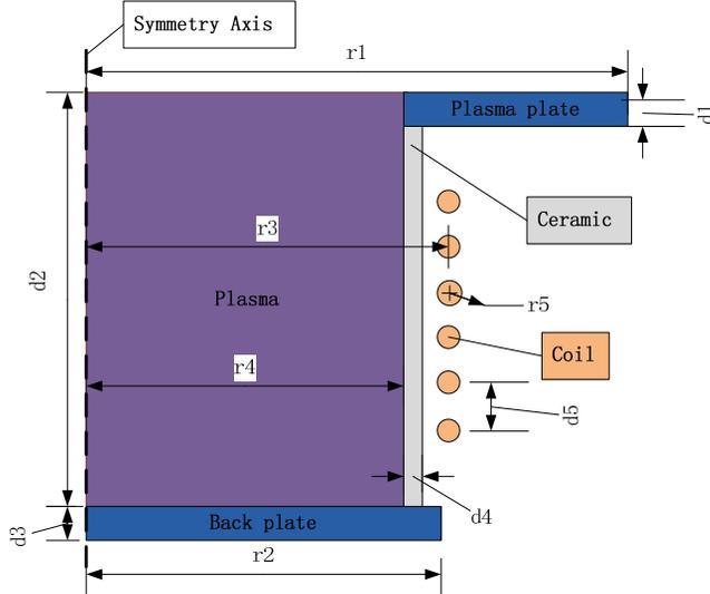
Figure 3: Schematic drawing of the FEM model.
