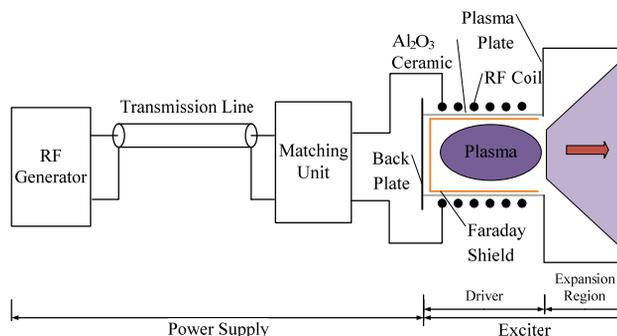
Figure 1: Schematic drawing of RF system of the exciter.
