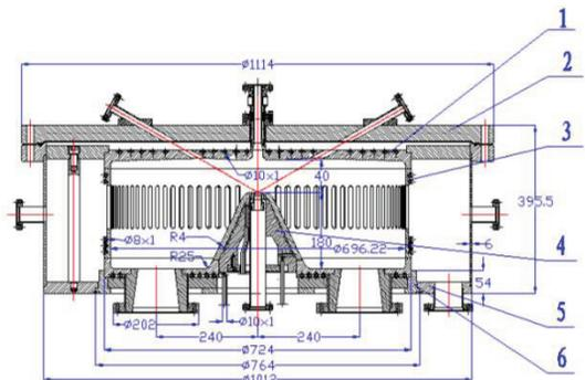
Figure 5: Mechanical design of the gun cavity proto-type.
