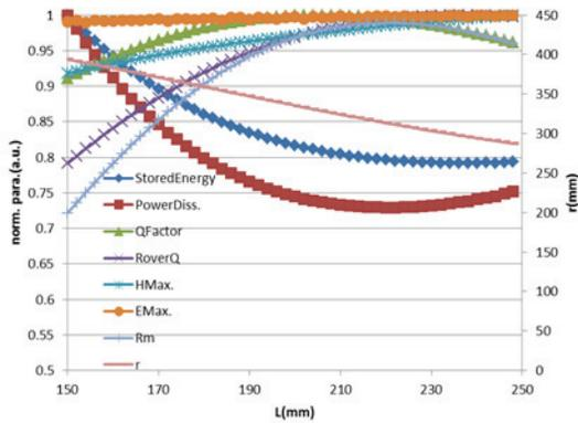
Figure 3: RF parameters of the cavity vs dimension of  $l$ .
