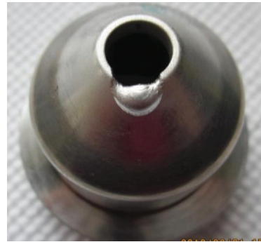
Figure 3: A photograph of the melt electrode heated by the dumping electrons.
