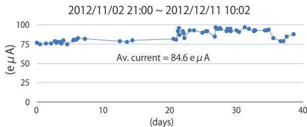
Figure 2: Beam intensity of U<sup>35+</sup> from the SC-ECRIS, measured in the LEBT of the RILAC2 during beam servicing in 2012.
