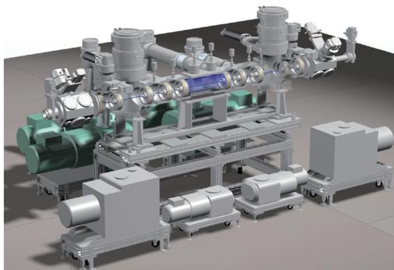
Figure 4: Schematic of helium gas stripper.
