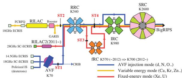
Figure 1: Accelerator chain of RIBF at RIKEN. Three injectors — AVF cyclotron, RILAC, and RILAC2 — are followed by the four booster cyclotrons — RRC (RIKEN Ring Cyclotron), fRC (fixed-frequency Ring Cyclotron), IRC (Intermediate-stage Ring Cyclotron), and SRC (Superconducting Ring Cyclotron). The K-values of the cyclotrons are indicated in the figure in MeVs. The charge strippers are indicated by labels in the red text (ST1 - ST4).
