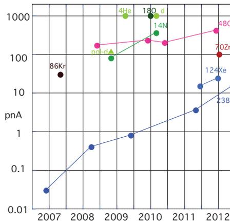
Figure 5: Evolution of maximum beam intensities at RIKEN RIBF.
