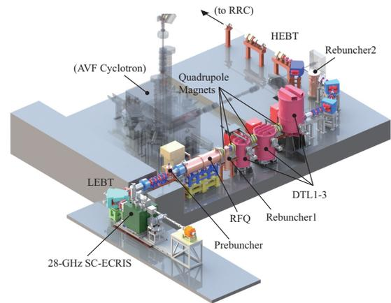
Figure 3: Schematic of RILAC2 injector.
