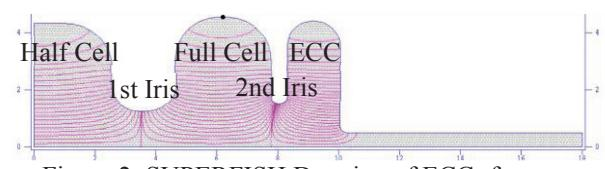
Figure 2: SUPERFISH Drawing of ECC rf gun.
