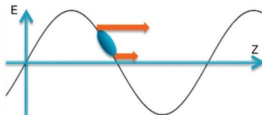
Figure 1: Off-crest rf phase acceleration in ECC.
