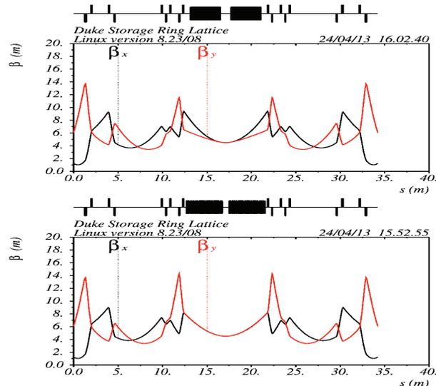
Figure 2: FEL straight section lattices with two different FEL wiggler configurations. Upper: with two planar OK-4 wigglers. Lower: with two helical OK-5 wigglers. In both cases, the central wavelength of the wigglers is set to be 450 nm with a 500 MeV electron beam.
