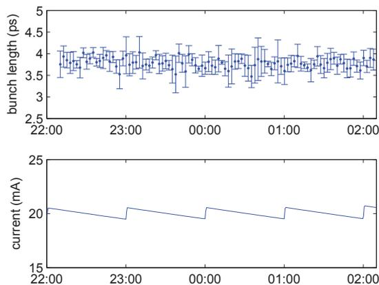
Figure 1: Bunch length data (top) and corresponding beam current (bottom) recorded for the short pulse mode (top-up) during February 2013.
