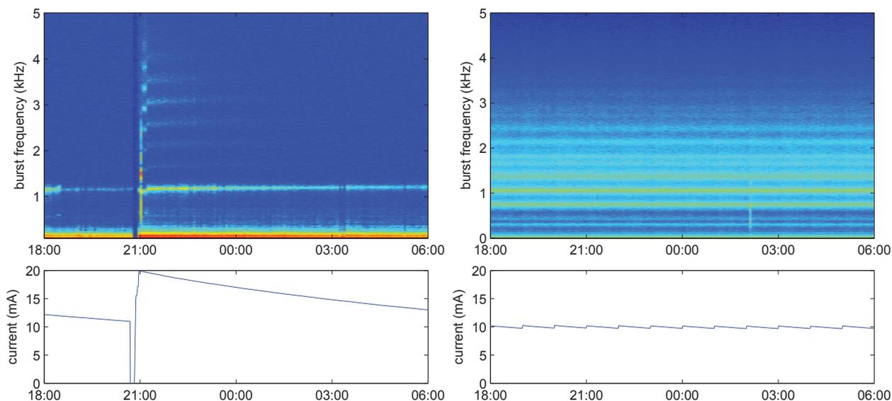
Figure 3: Spectrograms of temporal modulation in power recorded in the 60-90 GHz bandwidth using a Schottky Barrier Diode (top), along with beam current during the acquisition (bottom). The left hand images were recorded during decaying beam for the short pulse mode, and the right hand images show data recorded during top up operation in THz mode.
