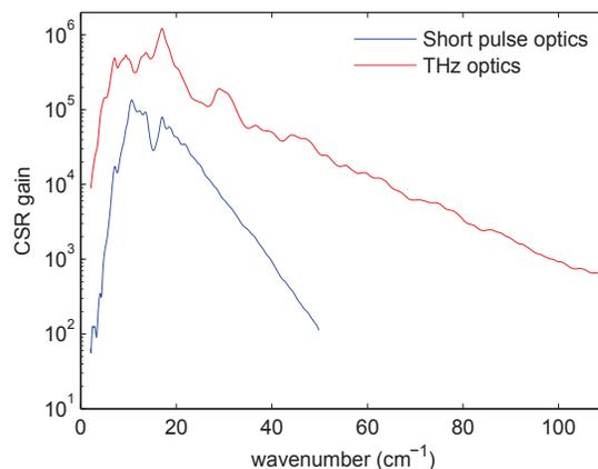
Figure 2: CSR amplification factors for the Short Pulse and THz modes (see Table 1). The CSR spectra were normalised using data recorded in standard user conditions, when 300 mA was stored in 686 bunches.
