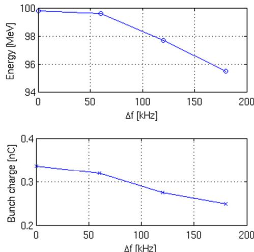
Figure 2: Effect of frequency change on linac performance.
