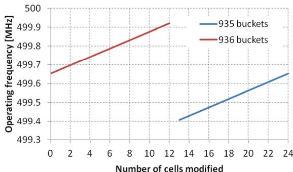
Figure 1: Frequency change required for multiple cell implementation of the DDDBA lattice.
