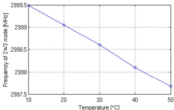
Figure 5: Temperature dependence of accelerating mode.
