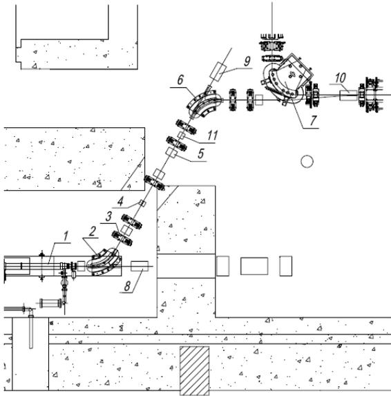
Figure 1: Layout of the NESTOR facility injection transportation channel: 1- linear accelerator, 2 – the first transportation channel dipole magnet, 3 – quadrupole lenses, 4 – collimator, 5 – dipole beam position correctors, 6 - the second transportation channel dipole magnet, 7 - the first storage ring dipole magnet, 8, 9 – scintillation screens and Faraday cups, 10 – inflector, 11 – beam current and beam position monitor.
