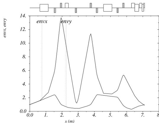
Figure 7: Transverse sizes of the beam along the beam transport channel in the stage 3.  $Envx$ ,  $Envy$  - horizontal and vertical beam size, respectively.
