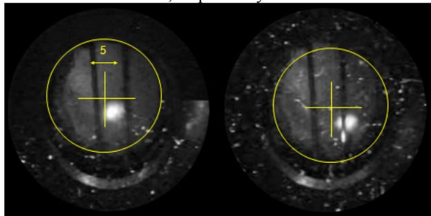
Figure 8: Focused beam at the inflector point with different forces of correctors (displacement of about 5 mm).
