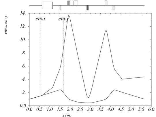
Figure 3: Transverse sizes of the beam along the transport channel in the second stage.  $em_{vx}$ ,  $em_{vy}$  - horizontal and vertical size, respectively.
