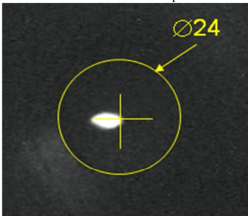
Figure 5: Electron beam shape behind the second bending magnet of the transport channel the (9, Fig. 1).
