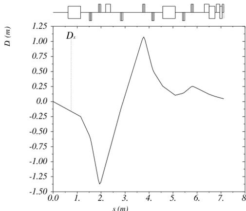
Figure 6: Dispersion function of the beam along the beam transportation channel at the stage 3.
