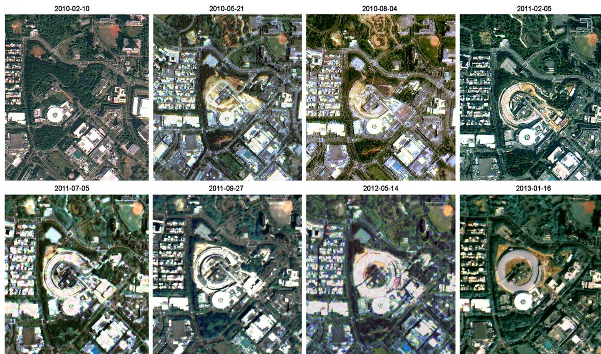
Figure 2: The satellite pictures show TPS civil construction progress in past years. The shortest distance between two circles across the intersecting point and SRF cavity, that is why the SRF cavity is so sensitive to the ground vibration of TPS civil construction.
