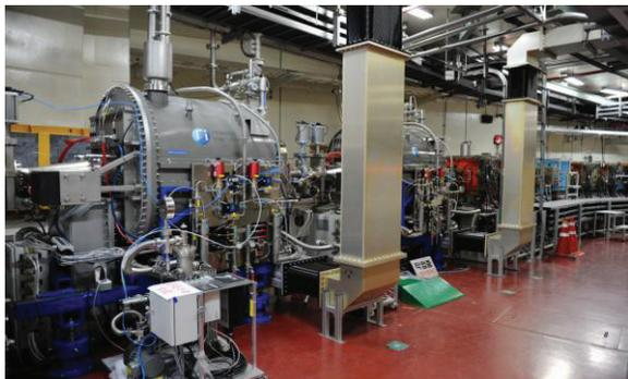
Figure 2: PLS-II SC RF cavities installed in the SR tunnel.
