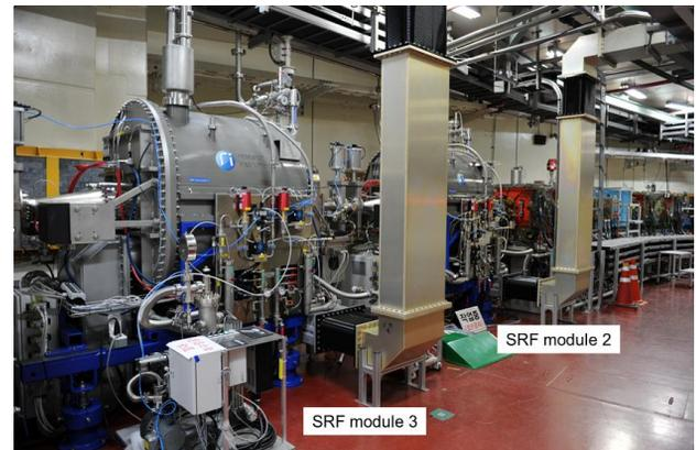
Figure 3: PLS-II RF system of phase-I (~2012).
