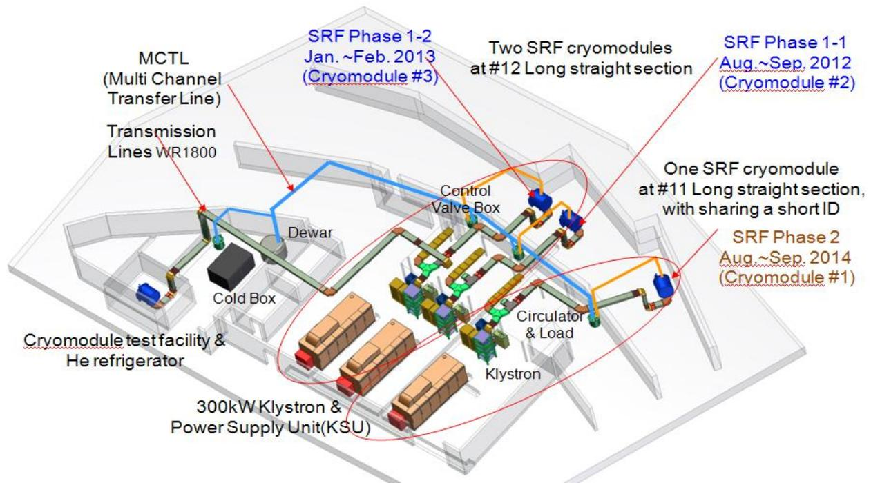
Figure 5: Layout of PLS-II RF system with three Cryomodules (phase-2).
