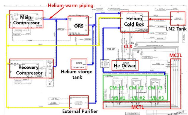
Figure 4: Block diagram of Cryogenic system.
