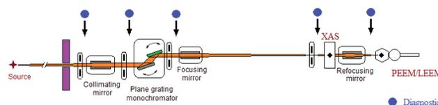
Figure 5: The conceptual layout of Solaris beamline.
