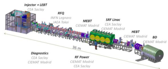
Figure 2: Layout of LIPAc and its construction sharing.
