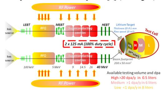
Figure 1: Schematic of IFMIF.
