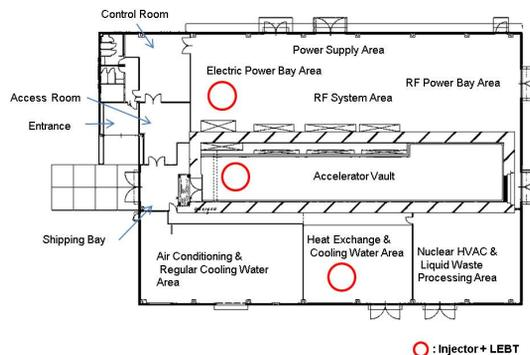
Figure 5: LIPAc complex building layout with indication of the position of Injector + LEBT related hardware.
