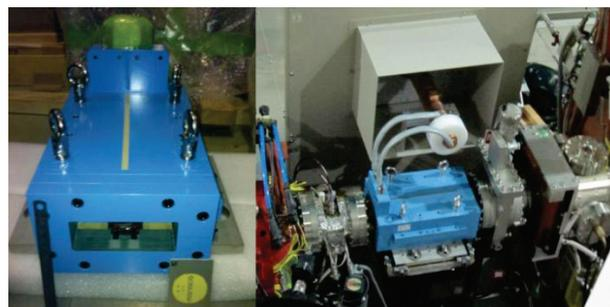
Figure 5: Photo of the pulse sextupole magnet.
