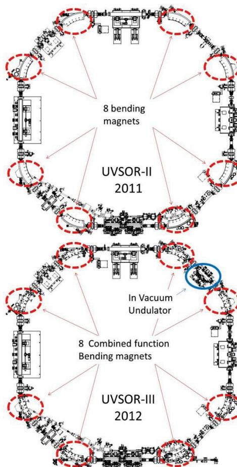
Figure 1: Layout of UVSOR-II (up) and UVSOR-III (down).
