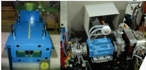
Figure 5: Photo of the pulse sextupole magnet.
