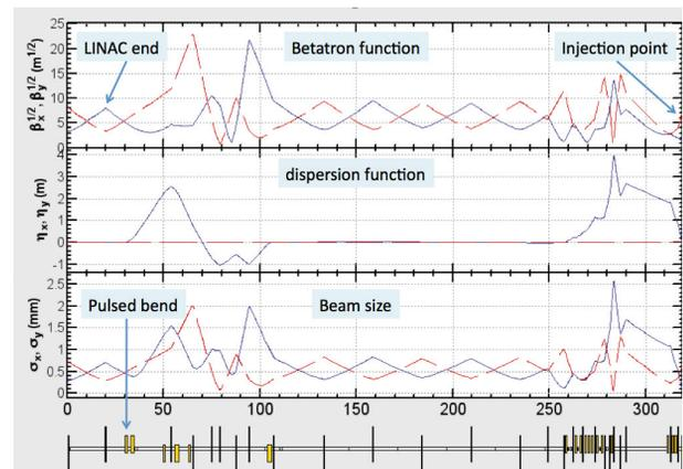
Figure 6: Optics from the end of the KEK LINAC to the injection point of the PF-AR. Blue and red lines represent the horizontal and vertical parameters, respectively.
