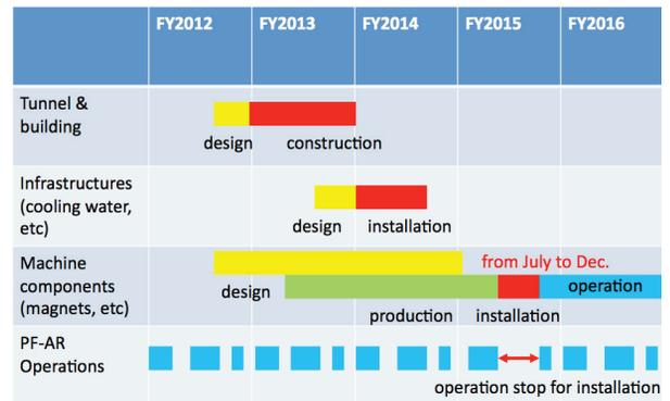
Figure 5: Construction Schedule of the PF-AR new transport line.
