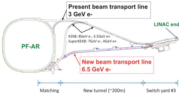
Figure 4: New beam transport line (red) for the PF-AR. A black line show the present beam transport line. A blue area is a new tunnel.
