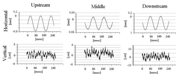
Figure 2: Example of the beam position measurement by the fast BPMs at the bump.
