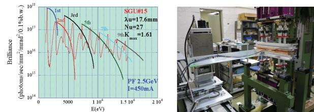
Figure 3: Calculated spectrum of the SGU#15 and a photograph of the SGU#15 during the magnetic measurement.
