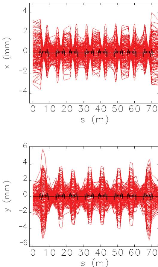
Figure 1. Distorted closed orbit in a super period of the storage ring for 200 seeds random errors, horizontal orbit (top), vertical orbit (bottom).
