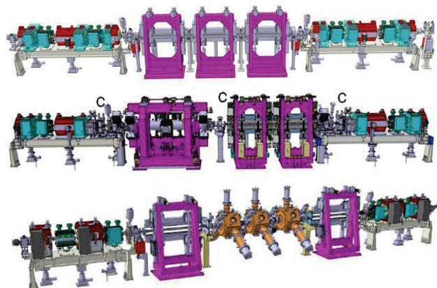
Figure 2: Standard 5 metre [Top], 6 metre ID16 [middle], 7 metre ID23 [bottom] straight sections.
