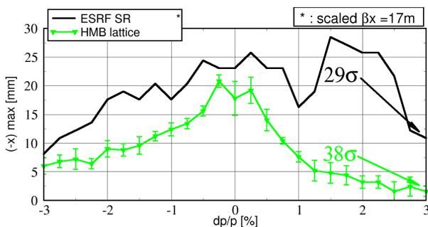
Figure 2: Dynamic aperture of the new lattice compared to the present one.
