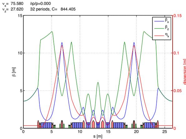
Figure 1: Optical function in the standard cell.
