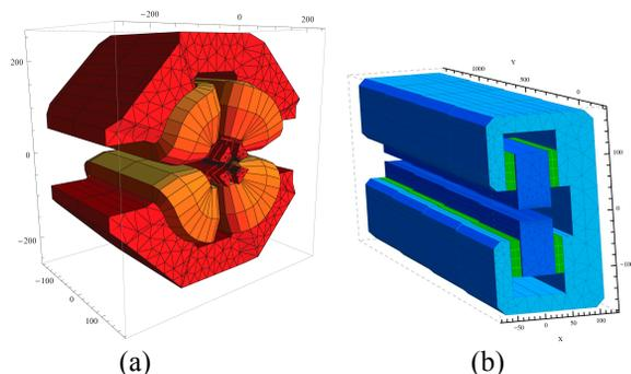
Figure 3: Magnetic design of a 100 T/m quadrupole prototype (a) and of a permanent magnet dipole with longitudinal gradient (b).
