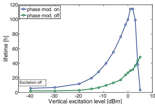
Figure 2: Beam lifetime as function of vertical excitation level with and without RF phase modulation.
