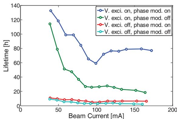
Figure 1: Beam lifetime as function of beam current with and without vertical excitation and RF phase modulation.
