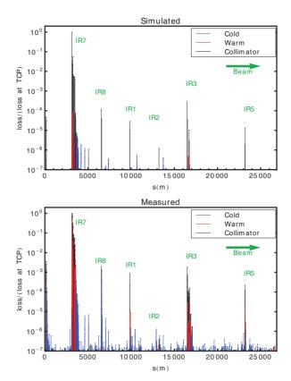
Figure 1: Simulated loss locations from SixTrack binned in 1 m intervals (top) and measured BLM signals from a qualification loss map on April 12, 2011 (bottom). The initial losses occur in both cases in the horizontal plane in B1.
