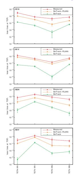
Figure 3: The ratio of BLM signal, or particles lost, on horizontal and vertical TCTs to the TCPs in simulations and measurements in the 2011 machine.
