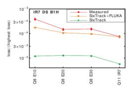
Figure 2: The ratio of BLM signal, or particles lost, at the BLMs with the highest signal in the IR7 DS, to the highest signal in the LSS, in simulations and measurements for the 2011 machine for horizontal losses in B1.
