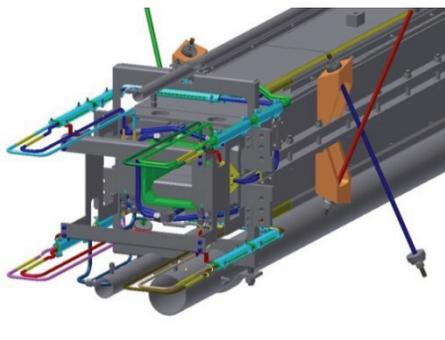
Figure 1: 3D view of the SIS100 FOS dipole cold mass.
