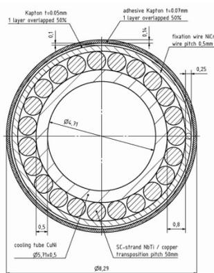
Figure 2: Cross section of the FOS cable.
