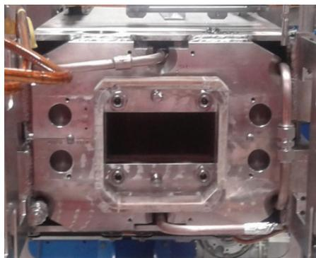
Figure 4: SIS100 FOS dipole cold mass.
