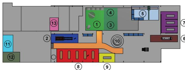
Figure 5: Manufacturing layout for SIS100 series production: 1 = winding, 2 = baking press, 3 = coil insulation, 4 = electric tests of coils, 5 = yoke stacking, 6 = yoke heat treatment, 7 = assembly half-yokes, 8 = assembly cold mass into cryostat, 9 = geometrical measurements, 10 = coil He leak test, 11 = pre-manufacturing of busbars, 12 = component leak test, 13 = thermal shield manufacturing
