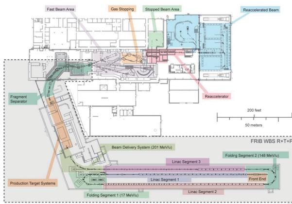
Figure 4: Layout of FRIB (hatched area) at MSU.
