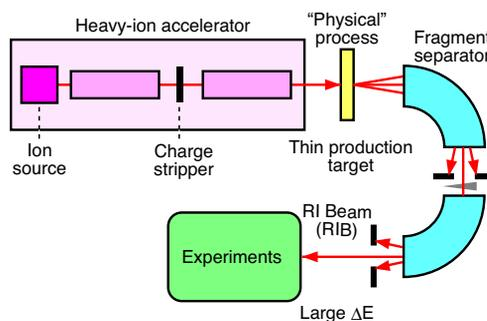
Figure 1: Schematic drawing of the in-flight production method.
