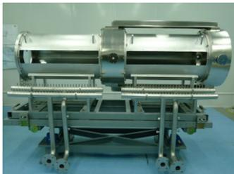
Figure 14: RCS cavity in mass production.
