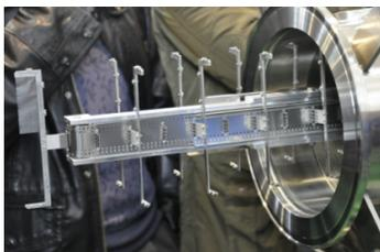
Figure 15: Stripping foil for  $\text{H}^-$  injection.
