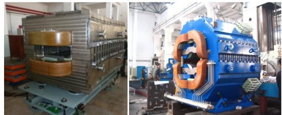
Figure 13: RCS dipole and quadrupole prototype magnets in mass production.
