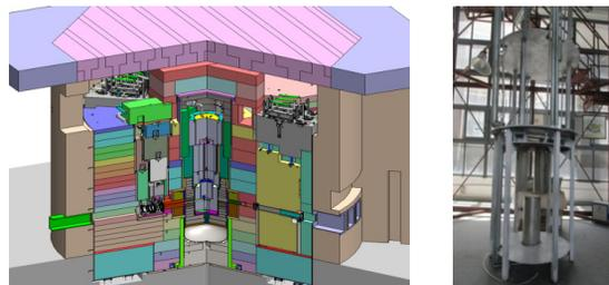
Figure 16: Target-moderator-reflector design and its maintenance mock-up.
