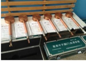
Figure 10: The fabricated drift tubes.
