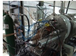
Figure 5: CSNS H<sup>-</sup> ion source in beam extraction test.
