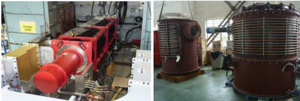
Figure 11: 3MW klystron and its 120 kV HVPS under manufacture.
