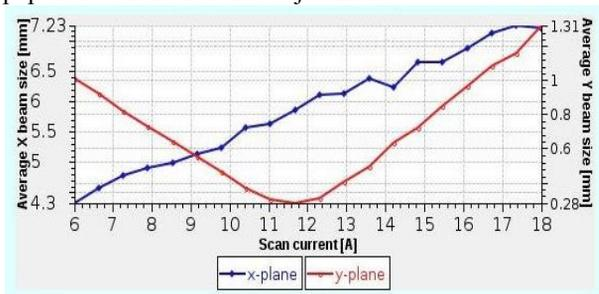
Figure 4: Vertical Emittance measurement in single bunch mode. The plot is rms beam size in the flag immediately upstream of the first dump vs. the LB-Q1 quadrupole current.
