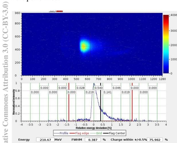
Figure 2: The energy spread measurement at flag LB-VF2 in Multibunch Mode. This is a beam image of a 11nC bunch train. The horizontal beam size is 3.5mm FWHM, corresponding to a 0.41% FWHM energy spread.
