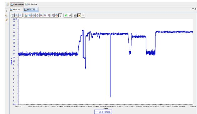
Figure 3: Multibunch Mode charge measured on ICT, LB-IT1. The horizontal axis spans 45 minutes. The vertical scale is train charge. After an initial level of 12 nC, the linac is tuned so 18nC exits the linac.
