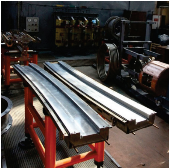
Figure 2: Halves of the yoke of the NICA booster dipole magnet before assembly of its winding.
