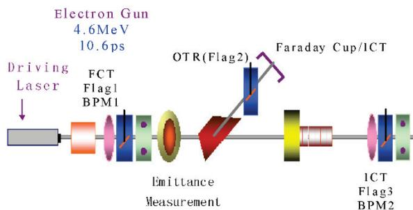
Figure 1: Original beam diagnostic system of RF gun.
