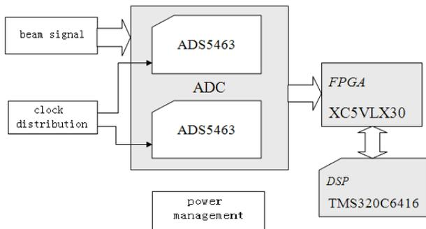
Figure 5: Sketch of high speed data acquisition system for cavity-based multi-parameter beam diagnostics.
