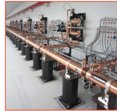
C-band high gradient acceleration system
