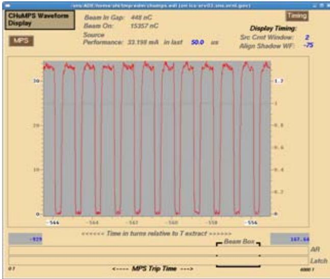
Peak Current Distribution in Minipulses for "30 mA" Beam
