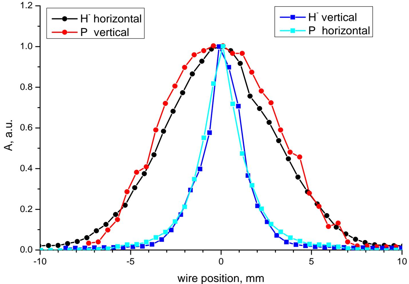
Vertical and horizontal planes are switched for protons in HEBT
