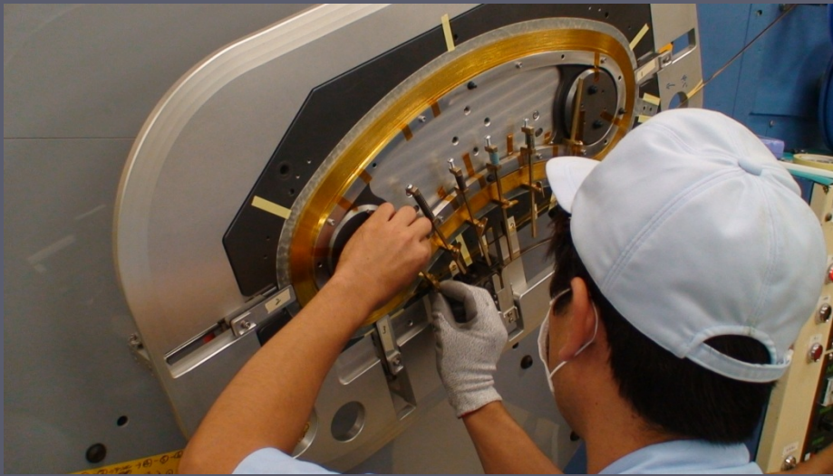
Double pancake (DP) was wound applying tensile stress.
