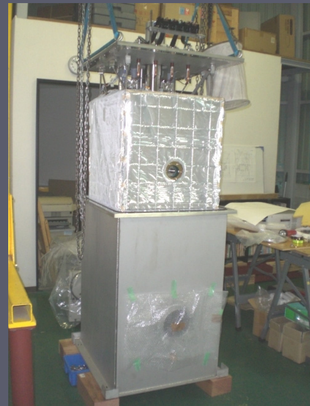
Installation into the cryostat.
