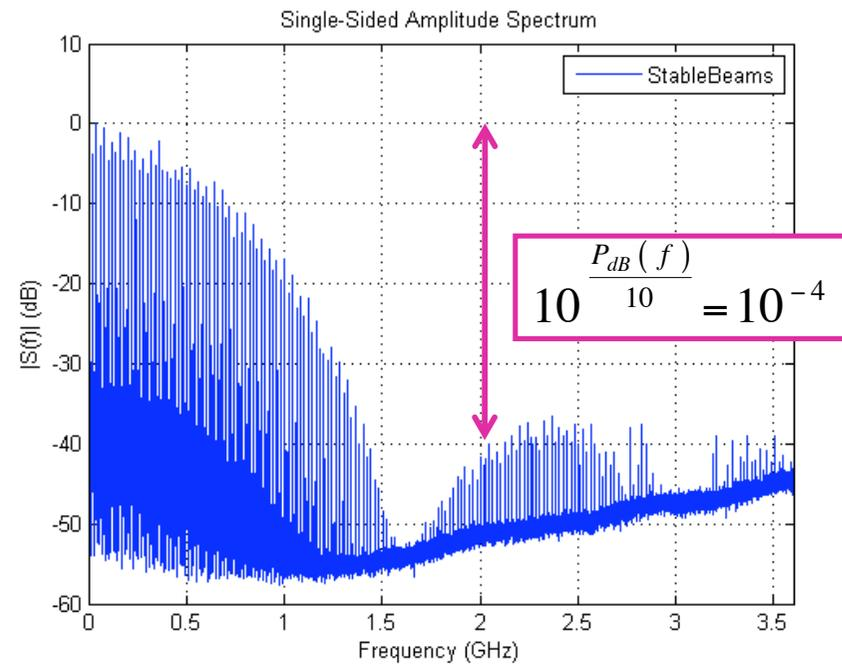
Coupled-bunch lines spaced by  $M f_0 \sim 20$  MHz (for 50 ns bunch spacing)  $\Rightarrow$  It would be  $\sim 40$  MHz for 25 ns
