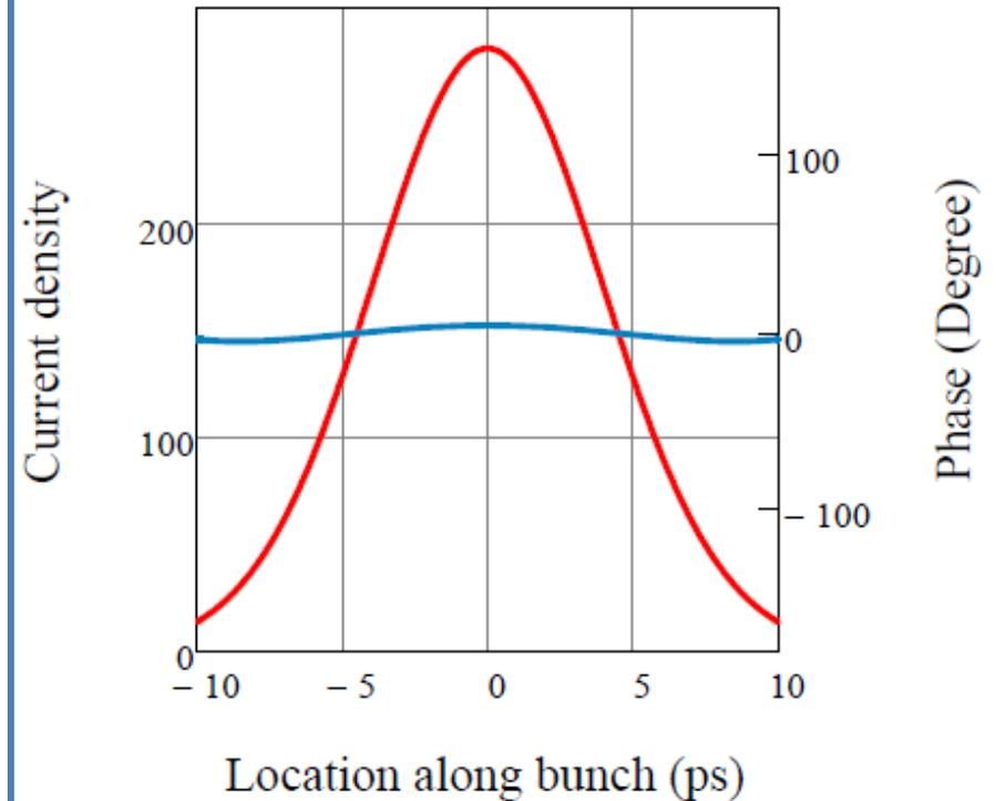
Increasing bunch length from 5 ps to 8.3 ps, and increasing bunch charge from 1nC to 1.67 nC reduces the phase shift across the bunch to less than 4 degrees with slightly reduced gain at the center slice.
