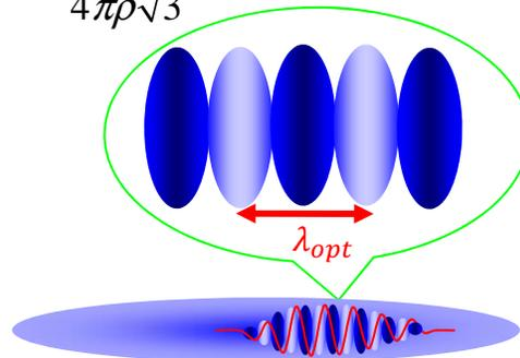
**Free Electron Laser (FEL):** The FEL amplifies the electron beam density modulation producing a series of pancakes spaced by the FEL wavelength
