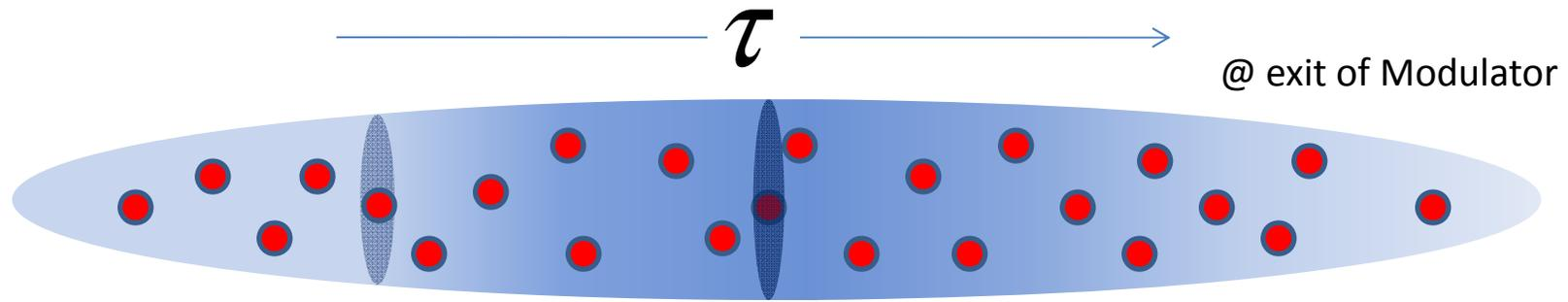
Due to charge density and average energy variation along the electron bunch, ions in off-center slices will not be put to the ideal position for cooling.
