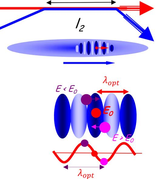
**Kicker:** Phase of the density modulation and corresponding longitudinal electric field in e-beam is adjusted in such way that it decelerate hadrons with higher energies and accelerate hadrons with lower energies. The resulting energy spread is reduced and the hadron beam is cooled.
