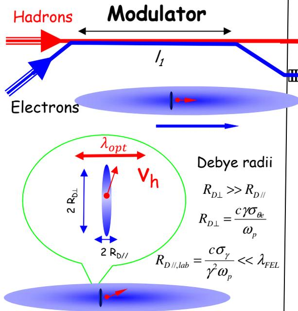
**Modulator:** Each hadron attracts a cloud of electrons creating a pancake-like modulation of the electron beam density
